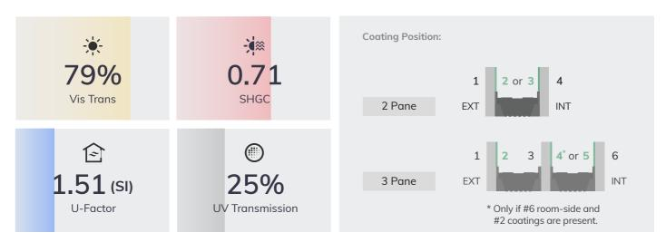
Data is produced using LBNL Window 7.8. 2-pane IG units have 13mm airspace and filled to 90% argon.
